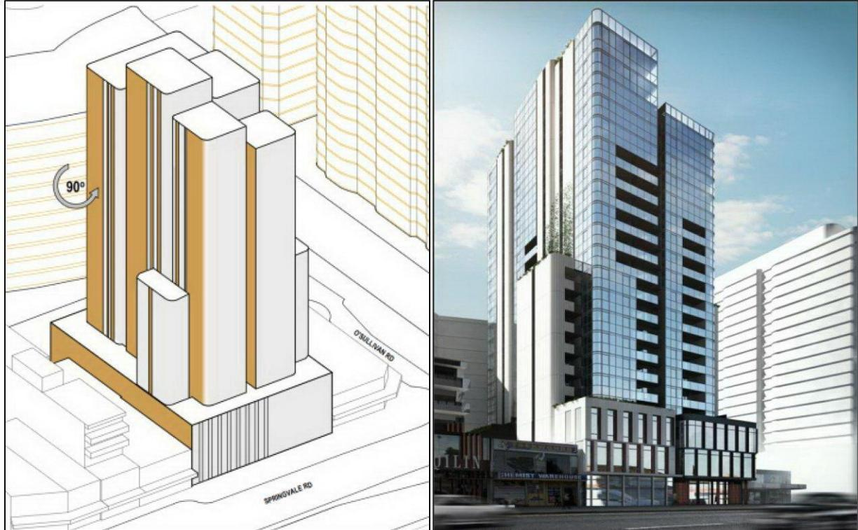
Figure 5- The proposed built form expressing the series of vertical clusters and platforms at various levels and how the proposed materials and finishes assist in defining these architectural elements. Source: *Plus Architecture*
