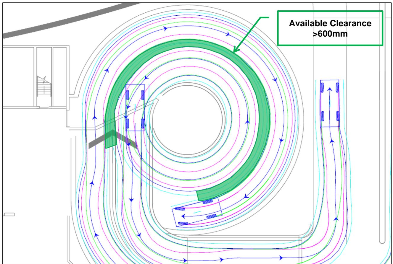
**Figure 1: Available Clearance on Circular Ramp**
