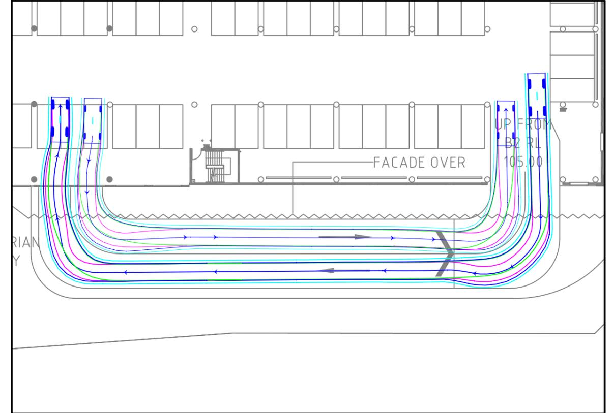
Eastern Ramp (Typical) - Autoturn IN and OUT
