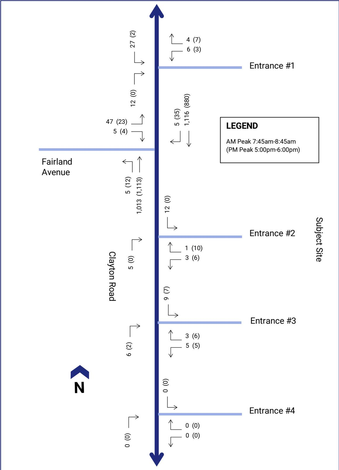
Figure 5: Turning Movement Counts of Existing Conditions
