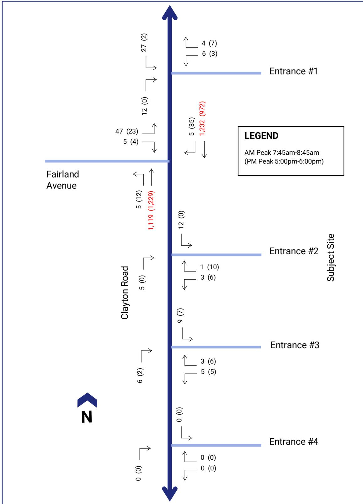
Figure 6: Turning Movement Counts of Existing Conditions – 10 year growth applied to Clayton Road (1% p/a)
