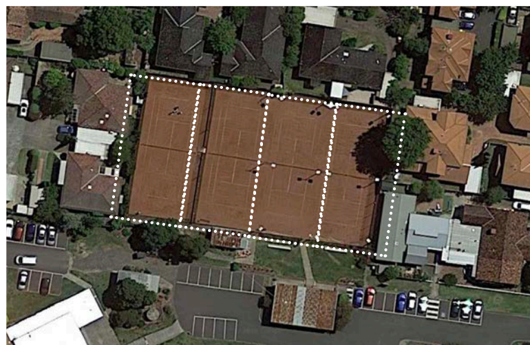
Existing tennis court dimensions compared to Tennis Australia standard for club/recreation courts (34.77 x 17.07m)
