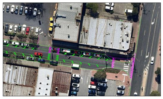
Figure 13: Indicative Diagram – Chester Street Reconfiguration (Aerial Source: Nearmap)
