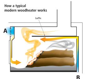
Primary air [A] is drawn in through a sliding or hinged air control mechanism, usually above the door. The air is preheated before being directed down the inside of the door, helping to keep the glass clean. It then enters the base of the fire. This primary air supply determines how guickly the firewood burns.
