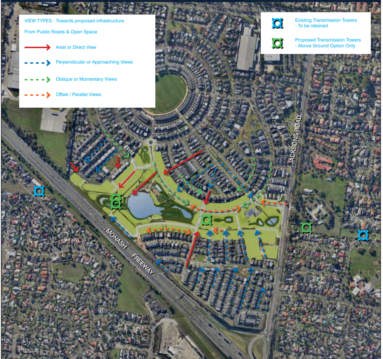
Figure 4 – Views towards Proposed Infrastructure - Above Ground Option
