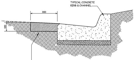
PROVISIONAL: CONSOLIDATED ASPHALT OF SIZE 10, TYPE N (CLASS 170) IN RESIDENTIAL ROADS TO SMOOTHLY MATCH TO EXISTING PAVEMENT LEVELS WITHOUT ANY DISCONTINUITY
