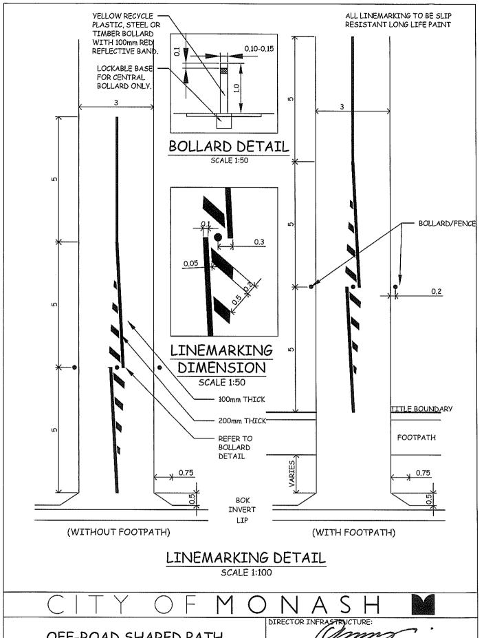
OFF-ROAD SHARED PATH PAVEMENT MARKING AND BOLLARD DETAILS DRAWN: RWL & SCALE: AS T.T.E MAR 2013 SHOWN
