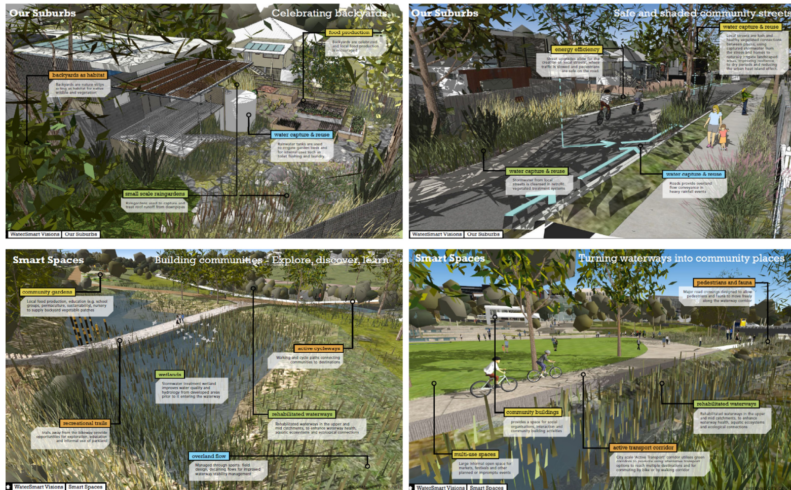
Figure 8: Water sensitive design at different urban scales (based on a presentation of the conference paper by Beardmore et al (2012) 13
