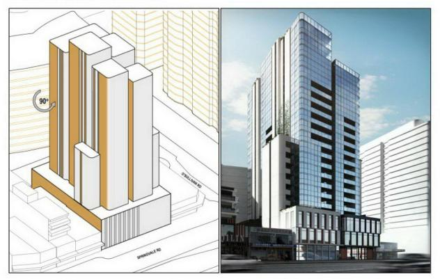
Figure 5– The proposed built form expressing the series of vertical clusters and platforms at various levels and how the proposed materials and finishes assist in defining these architectural elements. Source: *Plus Architecture*
