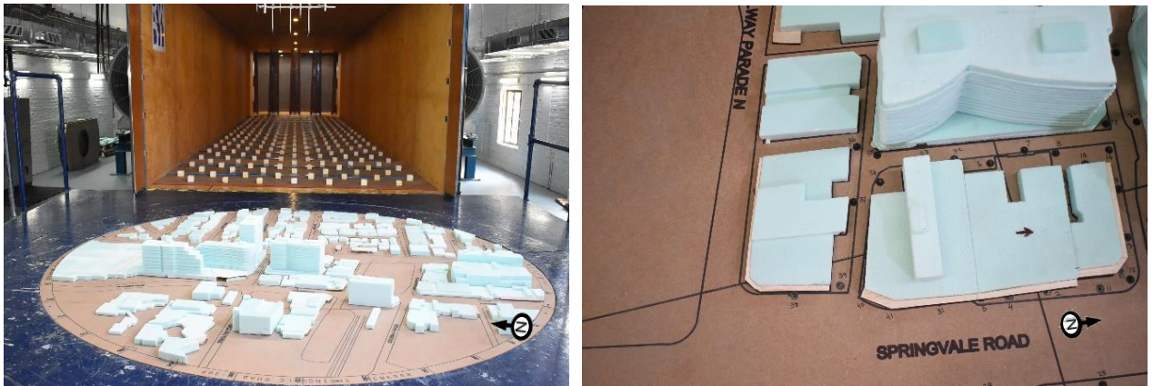
Image 2A: Wind Tunnel Study Model - Existing Configuration
