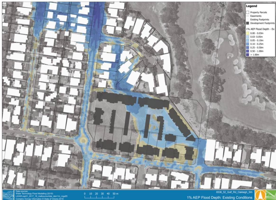
Figure 1-3 1% AEP Flood Depth – Existing Conditions
