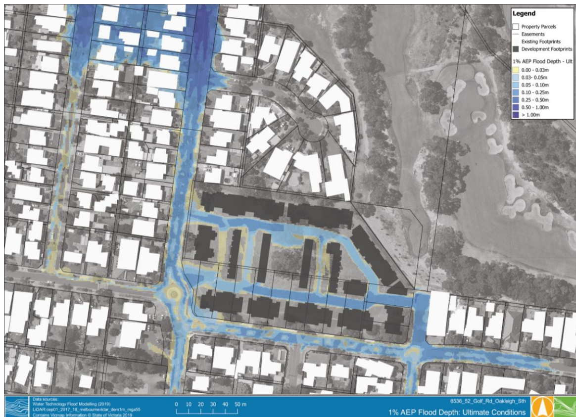
Figure 1-4 1% AEP Flood Depth – Ultimate Conditions
