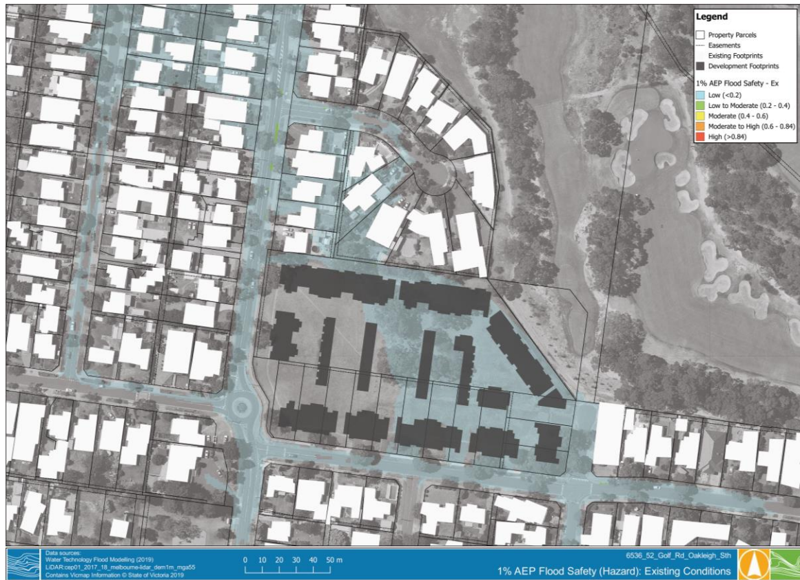
Figure 1-6 1% AEP Flood Safety (v.d ratio) – Existing Conditions
