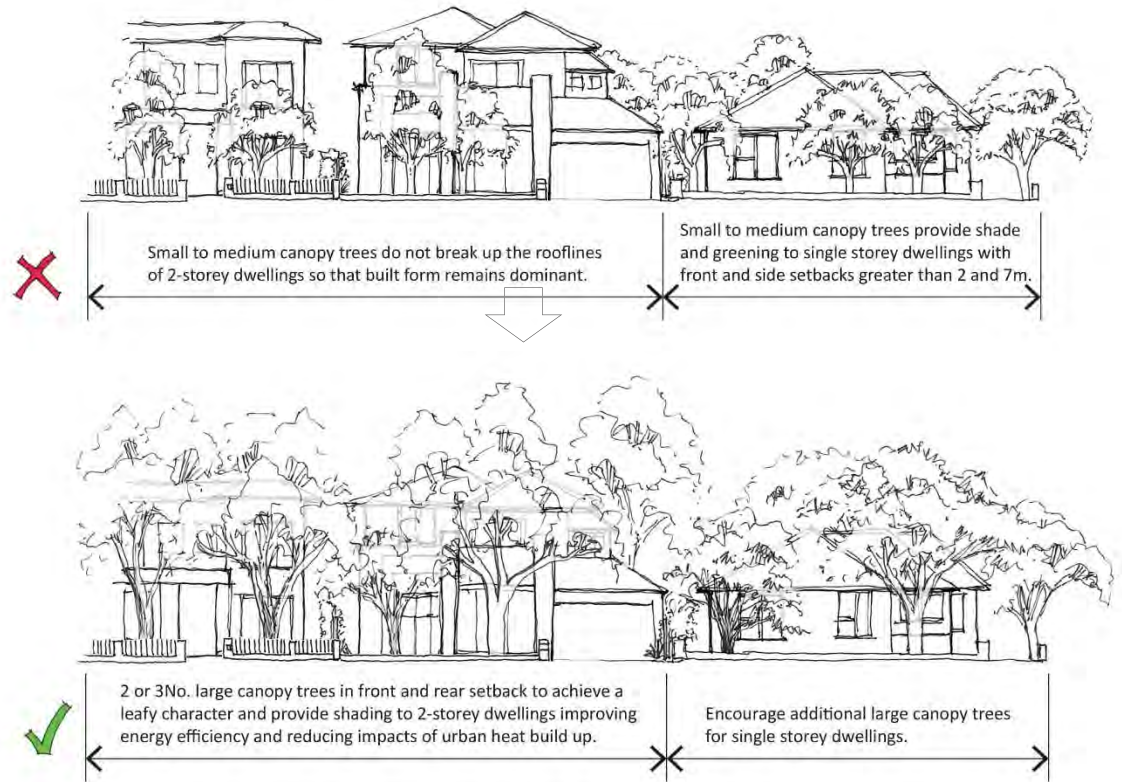
Figure 6A Preferred front setback with minimum 60 per cent grassed and planted surfaces
