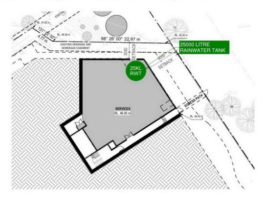
Figure 3.8 Proposed rainwater tank location within basement services plant area
