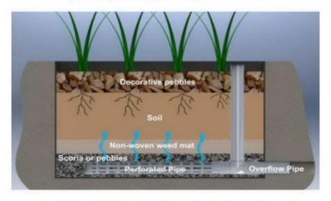
Figure 3.3 Typical Raingarden in ground for illustration purpose
