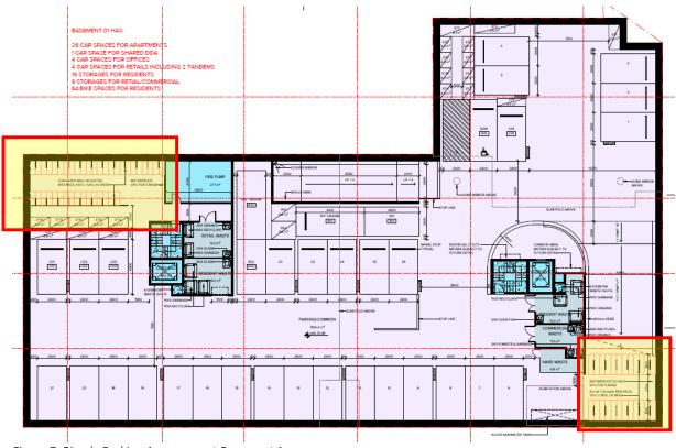
Figure 7: Bicycle Parking Arrangement Basement 1
