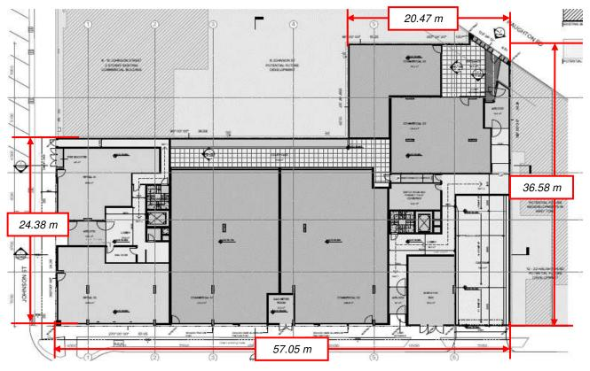
Figure 5: Ground floor plan with the plan-form dimensions overlaid.
