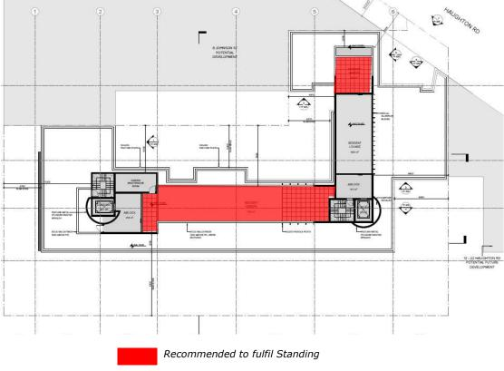
Figure 9: Roof Plan with recommended wind criteria overlaid
