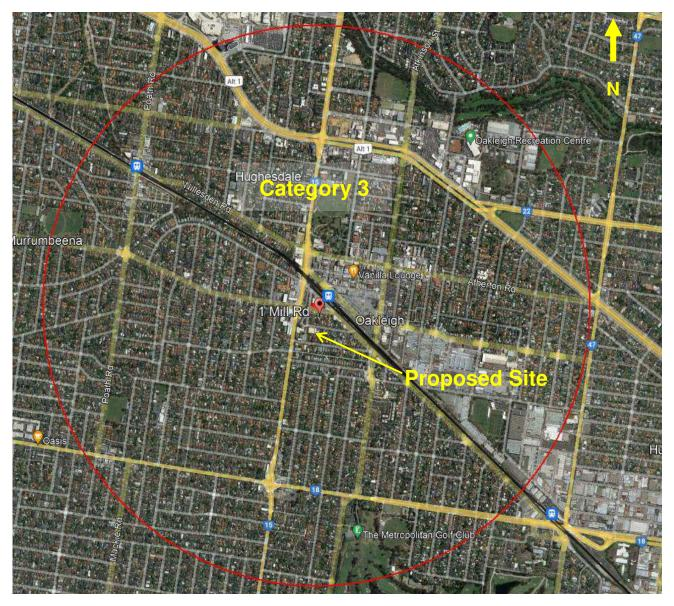
Figure 3: Assumed terrain categories for wind speed estimation.
