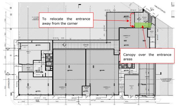
Figure 10: Ground floor plan with the recommended wind control measures overlaid
