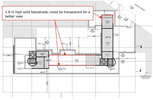
Figure 11: Roof plan with the recommended wind control measures overlaid
