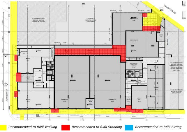
Figure 8: Ground floor with recommended wind criteria overlaid
