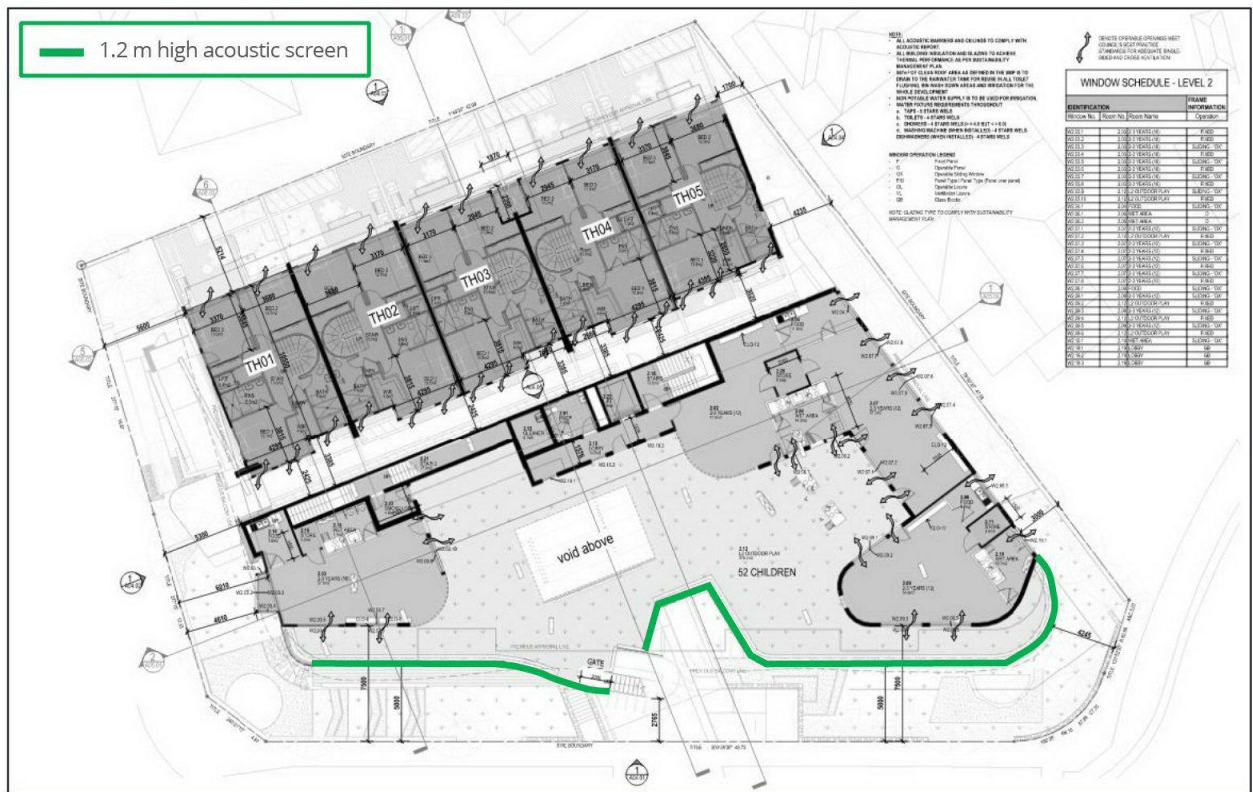
Figure 5 - Acoustic mitigation to ELC Level Two
