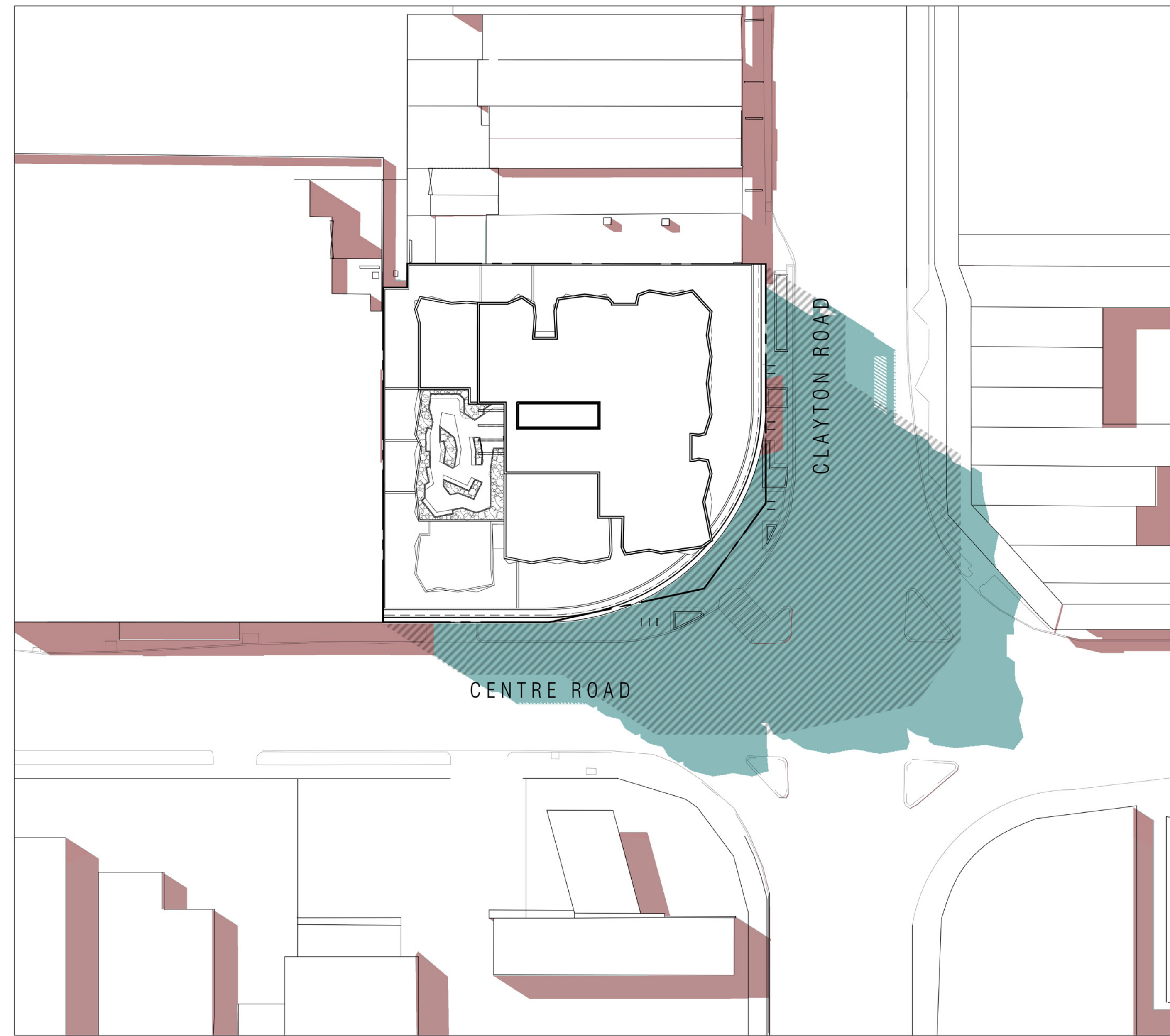
COMPARISON SHADOW DIAGRAM - 2PM, 22ND SEPTEMBER ■ EXISTING ■ PROPOSED ▨ 10 STOREY ENVELOPE IN LINE WITH CLAYTON PRECINCT PLAN
