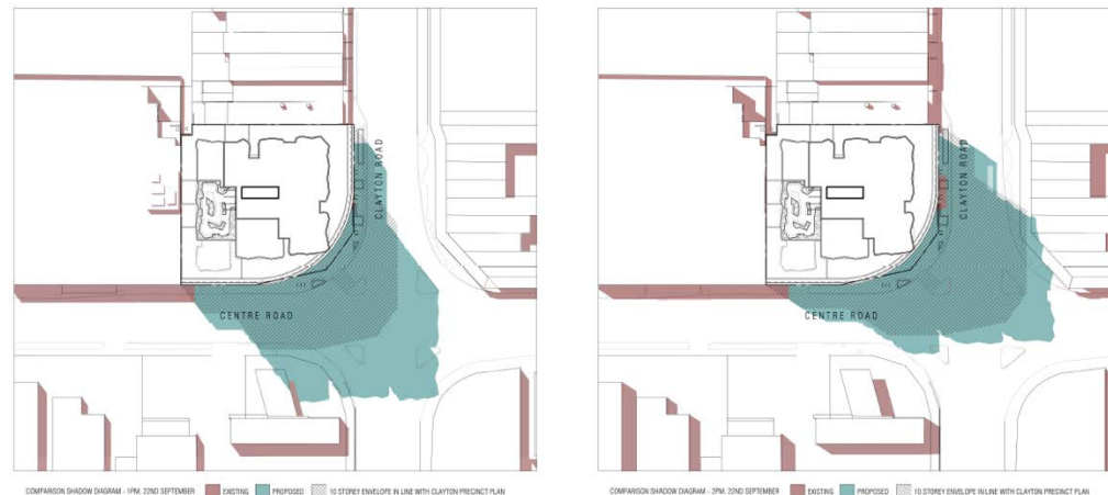
Figure 29: Shadow Diagrams between 1pm and 2pm at the equinox, prepared by Ewart Leaf
