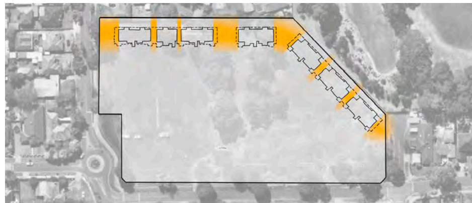
Figure 36 Breaks at first floor level provides visual transparency and minimises visual bulk
