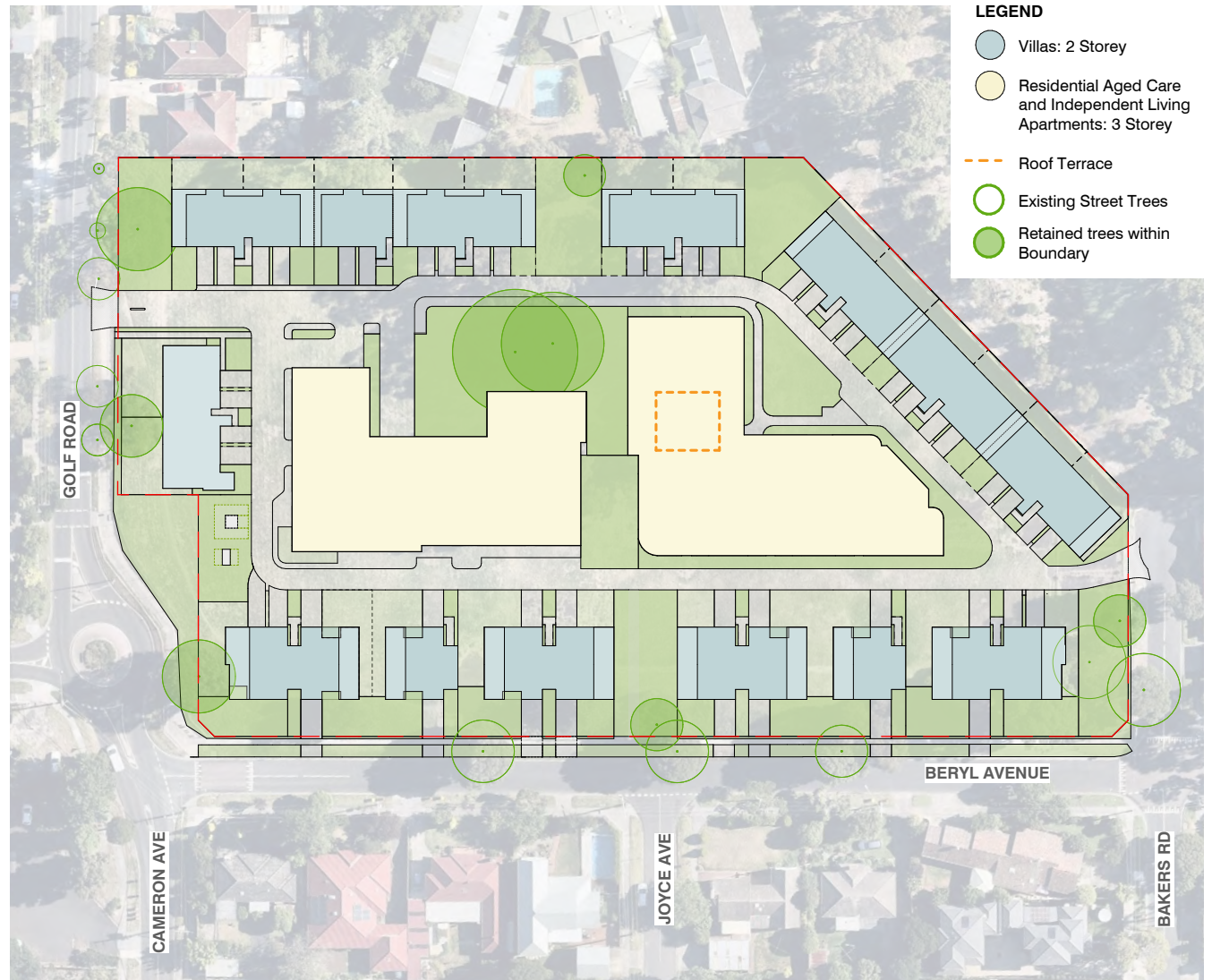
Figure 32 Building Heights and Setbacks
