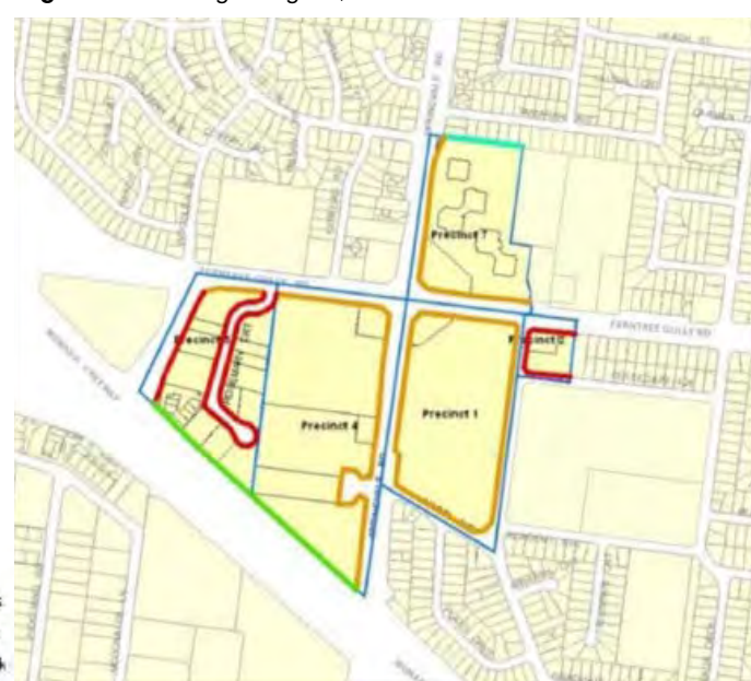
Figure 10 Building setbacks, DD08 Schedule 8
