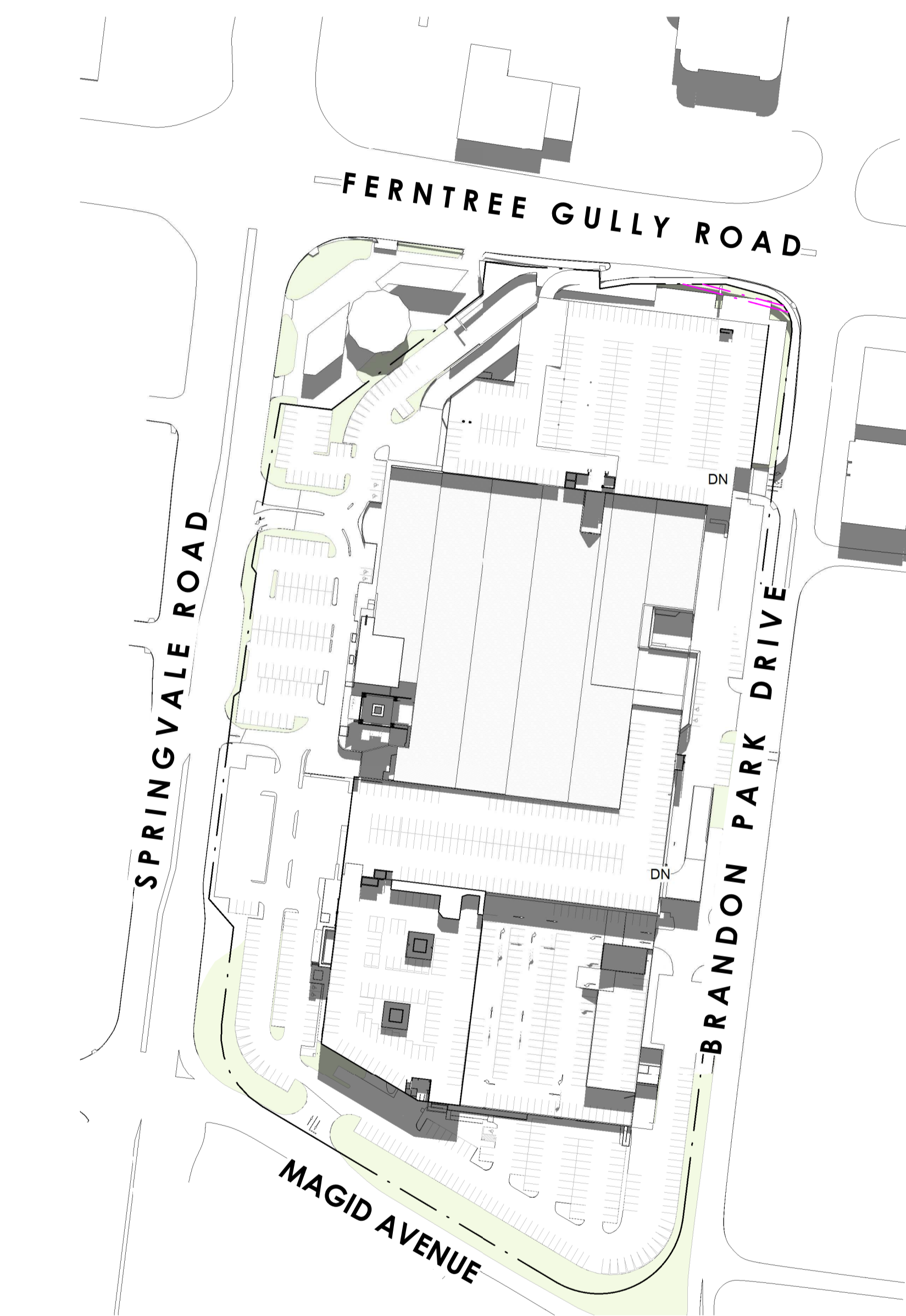
2 EXISTING SHADOW DIAGRAM - 22nd June 12pm Scale: 1 : 1500
