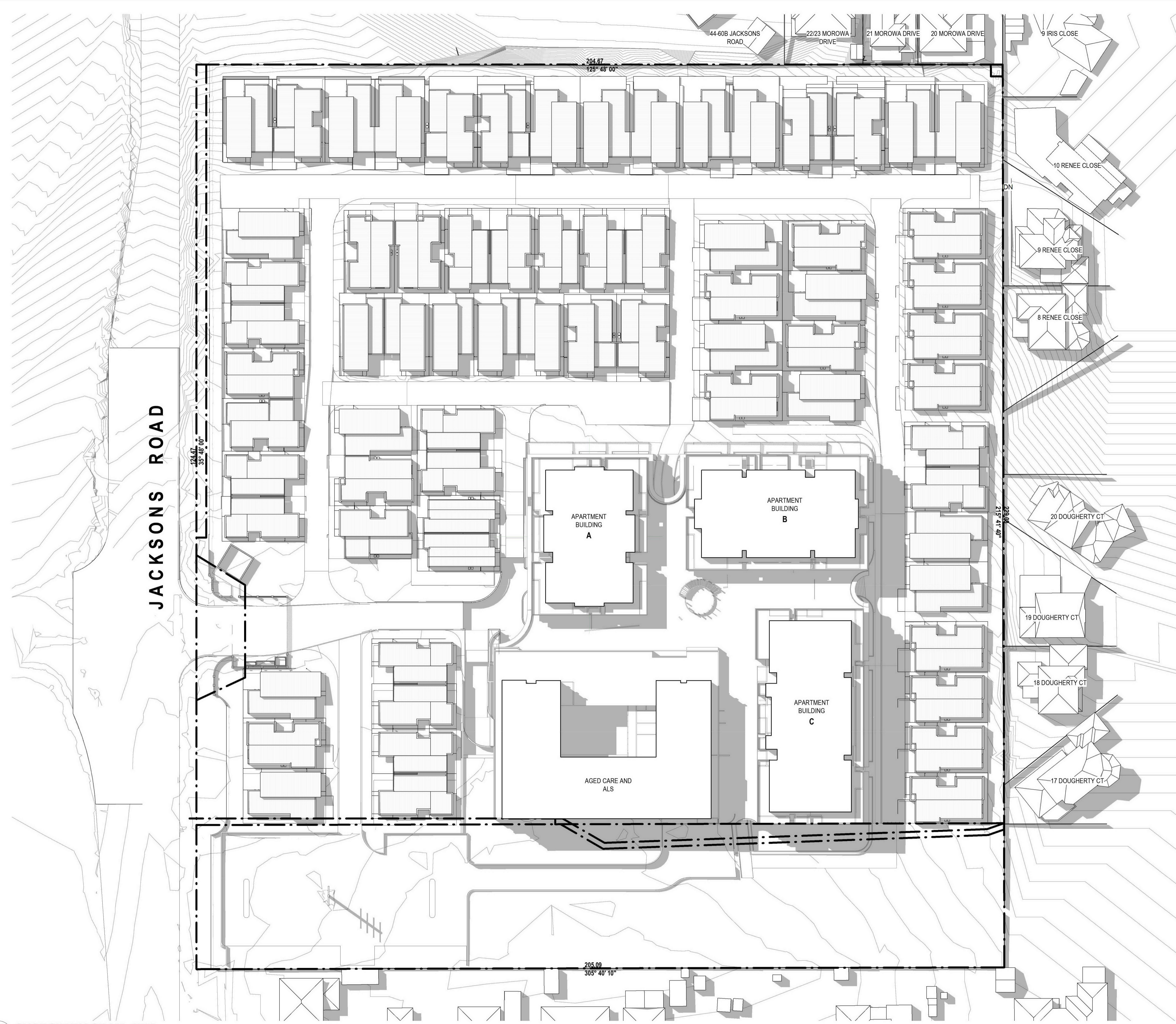
1 SHADOW DIAGRAM_2PM A1 sheet scale = 1:500
