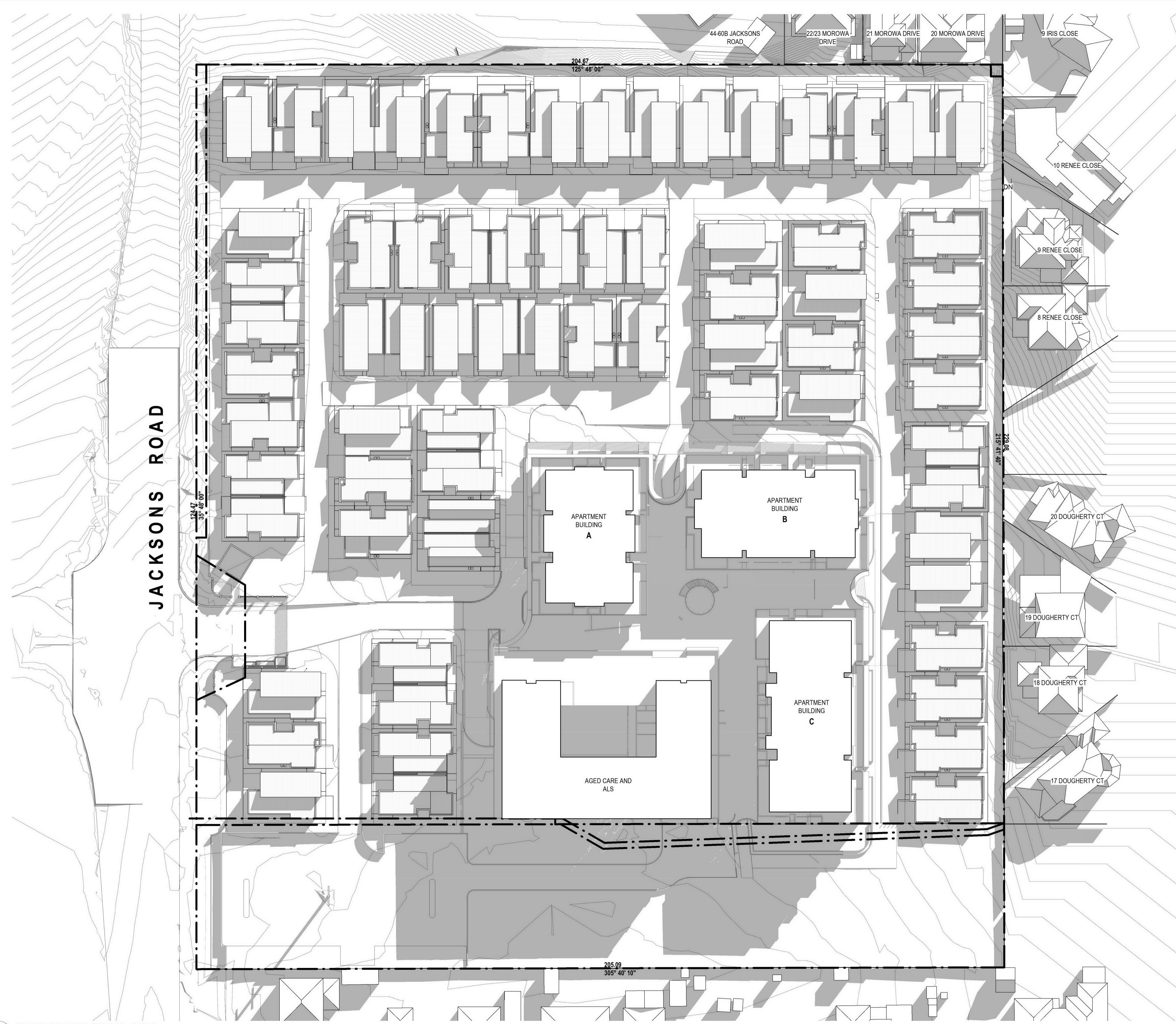
1 SHADOW DIAGRAM_9AM A1 sheet scale = 1:500
