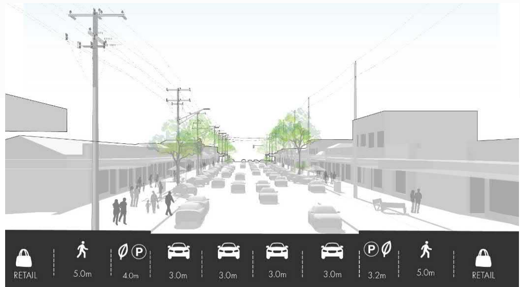
Figure 18. Clayton Road Existing Cross Section
