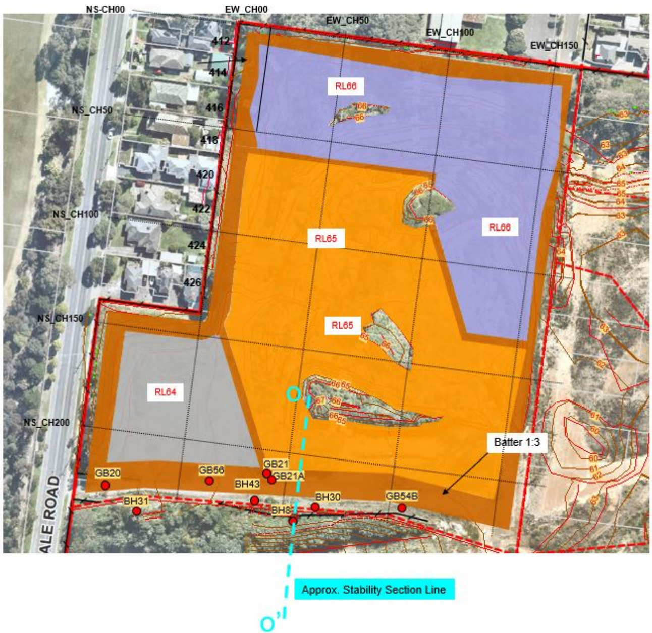
Figure D1 – Domain 1 proposed preload extending to the crest of the Domain 4 north batter
