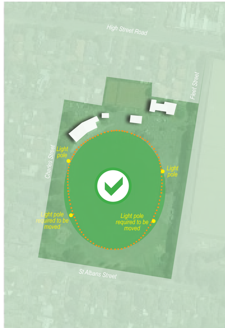
Option B Retain the existing oval location and size, but making modifications to remove the current 'egg' shape. The proposal shown is to reshape the southern part of the oval, which would require the existing oval lighting to be moved. The oval perimeter fencing would also be upgraded (black powder-coated chain mesh), safety fencing behind goals and spectator seating.
